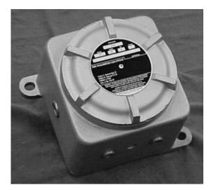
The SV-7 voltage adjuster is used for reducing supply voltage between 30-100VAC. This is standardly used for MI cable designs when full voltage exceeds application requirements.
