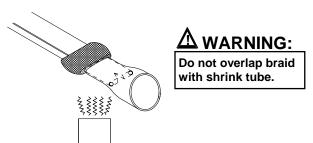
Slide a 51mm (2") length shrink tube over the heater cable leaving 25mm (1") of shrink tube past the heater cable. Shrink with heat gun until completely shrunk.
