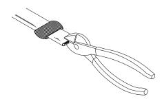
2 At the end of the heater cable, snip a 9.5mm (.375") slit between the bus wires. Slightly spread wires apart.
