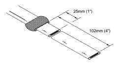
Out heater cable off at required length. Strip overjacket back 102mm (4") from the end of heater cable. Slide braid back over the overjacket portion of the heater cable. Cut off excess heater cable leaving 25mm (1").
