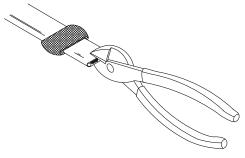
At the end of the heater cable, snip a 10mm (0.4") slit between the bus wires. Slightly spread wires apart.
