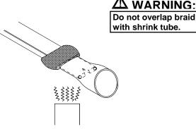
4 Slide a 13mm (0.5") diameter, 51mm (2") length shrink tube over the heater cable leaving approximately 25mm (1") of shrink tube past the heater cable. Shrink with heat gun until completely shrunk.
