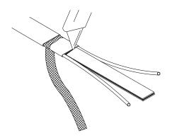
**6** Remove the exposed core material.
