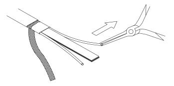
**5** Starting at the end, in the same plane as the cable, pull each bus wire away from the core material.
