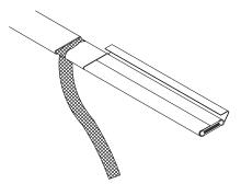
**3** Remove the jacket from the heater cable.
