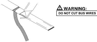
**4** Shave the core material from the outside of each bus wire.
