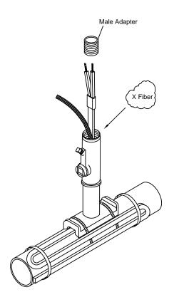
Note: If this kit is mounted in an orientation that would allow the sealing compound to flow out, place packing material (X Fiber) around the heater cable.
