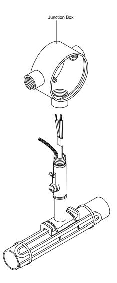
• Place junction box over the heater cable and braid, screw onto male adapter until secure.
