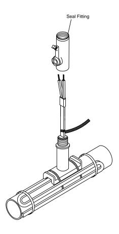
• Slide seal fitting over the heater cable and braid, screw onto the stand-off by hand until snug fit.
