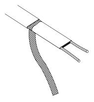
$\bullet$  Cut 6mm (0.25") off the end of each bus wire.
