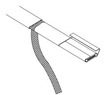
**3** Remove the jacket from the heater cable.
