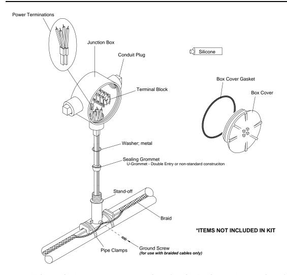
Note: This detail shows external grounding of braid. For internal grounding of braid (overjacket products), see sheet 8.
