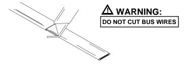
**4** Shave the core material from the outside of each bus wire.
