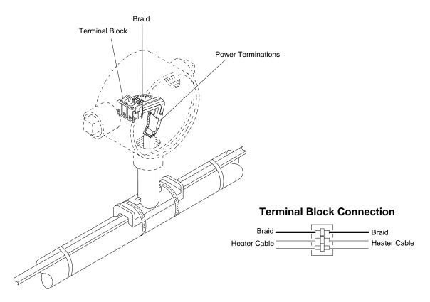
Note: This detail shows internal grounding of braid.
