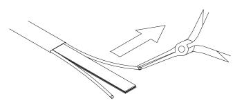
**S**tarting at the end, in the same plane as the cable, pull each bus wire away from the core.
