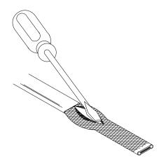
**5** At the bulge, separate the braid to make an opening.
