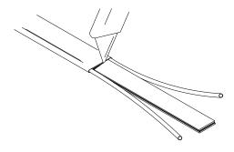
**6** Remove the exposed core material.
