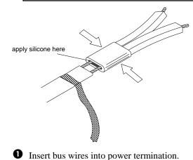
**2** Squeeze power termination opening and fill with
