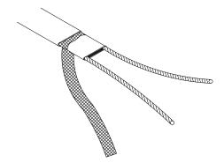
Cut 6mm (0.25") off the end of each bus wire.
