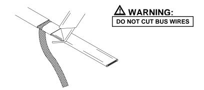
Shave the core material from the outside of each bus wire.
